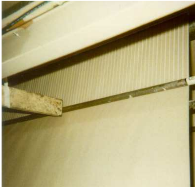
Photograph 1. Extrusion of Glue in Thin Lines onto Kraft Paper
